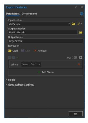
Make a new layer of the selected parcels by right clicking on the layer name in the Content pane and selecting Data > Export Features. The Output Location defaults to the project's default database. Give the new layer a meaningful name in Output Name.
